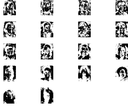
Figure 3. The 18 first eigenfaces for a set of 20 training images of size 82 \times 65 .
